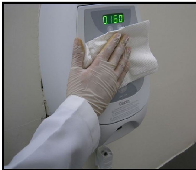
Figure 15. Electric controls should be disinfected by moisten towels
