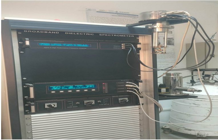
Figure 5. Broadband Dielectric Spectrometer (BDS) used for dielectric characterization (Source: Designed and produced by the authors).
